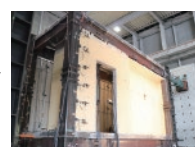
Real scale experiment of steel structure with non-structural components
