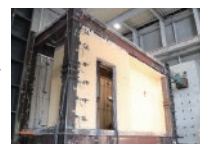
Real scale experiment of steel structure with non-structural components
