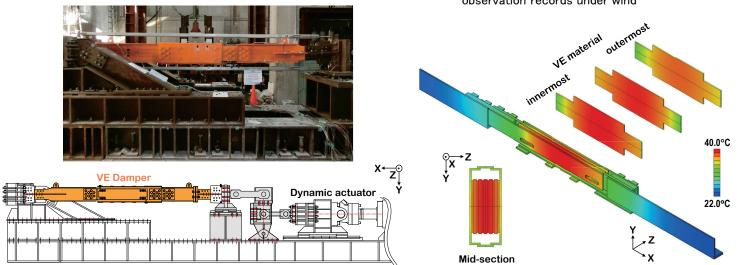
Experimental and analytical investigations of full-scale multi-layered viscoelastic damper under long-duration excitations
