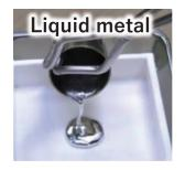
Various high-performance liquid metal coolants (Pb, Pb-Bi, Li, Pb-17Li, Sn, etc.) are currently being researched in our laboratory for use in fast and fusion reactors worldwide. Experimental investigations of the synthesis and thermophysical properties of these materials are underway.
