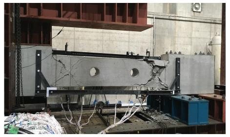
Loading test of RC beam with openings
