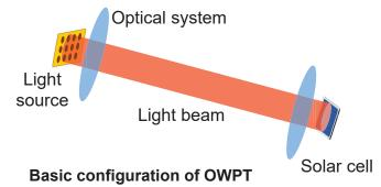
Consists of light source and solar cell, optical system for beam shape control, target detection, beam scanning, etc.
