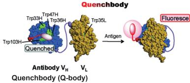
Fluorescent biosensor based on the antigendependent removal of a quenching effect on a fluorophore attached to antibody domains. This sensor is expected to have a range of applications, from in vitro diagnostics, to imaging of various targets in situ. (©American Chemical Society)
