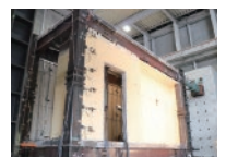
Real scale experiment of steel structure with non-structural components
