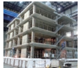
Shaking table test on real scale high performance RC buildings
