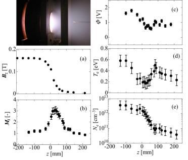
Supersonic acceleration and potential formation of arc-jet plasma along diverging magnetic field: Photo of the arc-jet along openfield line, and (a) longitudinal magnetic field, (b) ion Mach number, (c) space potential, (d) electron temperature and (e) electron density.
