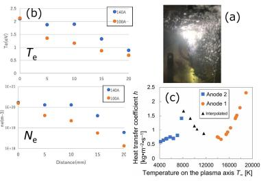
Arc-Jet in water for decommissioning of nuclear facilities: (a) Arc-jet ejected into water, (b) its electron temperature & density, and (c) heat transfer coefficient vs electron temperature on the plasma axis.
