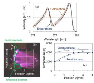
OES of  $N_2$  excited states of pulse-discharge plasma simulating automotive engines: (a) Theoretical fitting of  $N_2$  2PS spectrum in pulsed nitrogen plasma, (b) photo of the plasma and (c) position dependence of temperatures.
