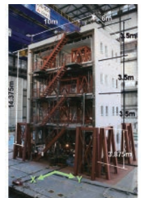
Full Scale Shaking Table Test of Steel Moment Resisting Frame
